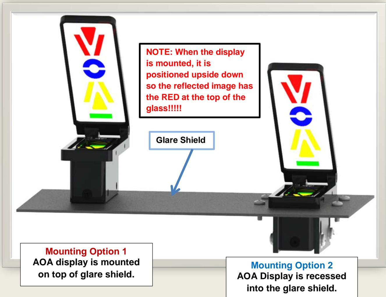
Most installations are completed as seen in **Option 2**. There must be 1.500” clearance under the glare shield to allow for the AOA case and the electrical cable clearance. The adjustable mounting brackets allow for thicknesses of glare shield and desired heights of the display mounting. To mount as seen in **Option 1**, there are two, 6-32 pre-threaded holes in the back of the display.
